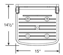
Seat width overall: 15" Seat depth overall:  $13^{1}/_{2}$ " Wall to front edge of seat:  $14^{1}/_{2}$ " Seat pad dimensions:  $13^{3}/_{4}$ "  $\times$   $10^{3}/_{4}$ "
