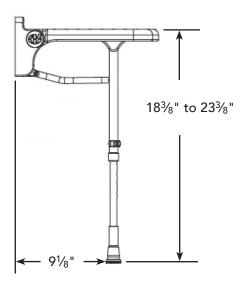
Seat width overall: 15" Seat depth overall:  $13^1/_2$ " Wall to front edge of seat:  $14^1/_2$ " Seat pad dimensions:  $13^3/_4$ "  $\times$   $10^3/_4$ "
