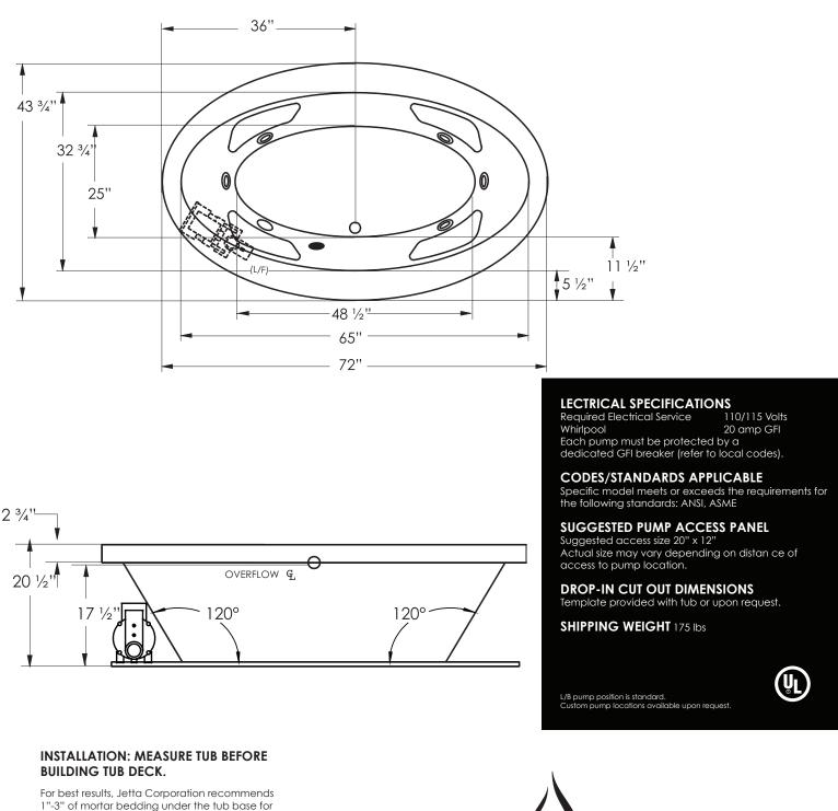
1"-3" of mortar bedding under the tub base fo maximum support. Contact Jetta for details. Dimensional variance on drawings may be +/-1/2 inch and are subject to change without notice.
