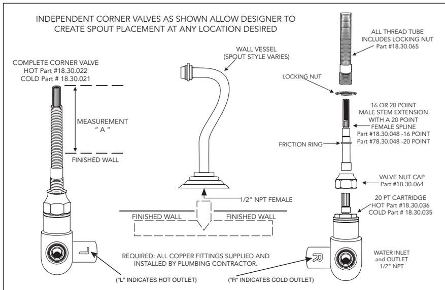
1. Rough-in Measurement A is from tip of valve stem to finished wall.
