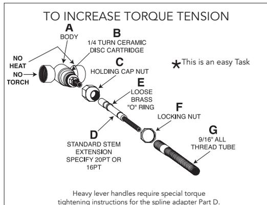
The design of our faucet allows the Qualified Plumbing Contractor to set the torque on each valve that uses the standard assembly B through G as shown (left) i.e. shut-offs - 2 valve - 3 valve, Pressure Balanced valves and all other valves with the above shown components. Note: Part E is a loose brass O-ring that is compressed inside Item G. The all-thread tube has a shoulder that through normal adjustment can be tightened or secured at the desired rate of the user.
