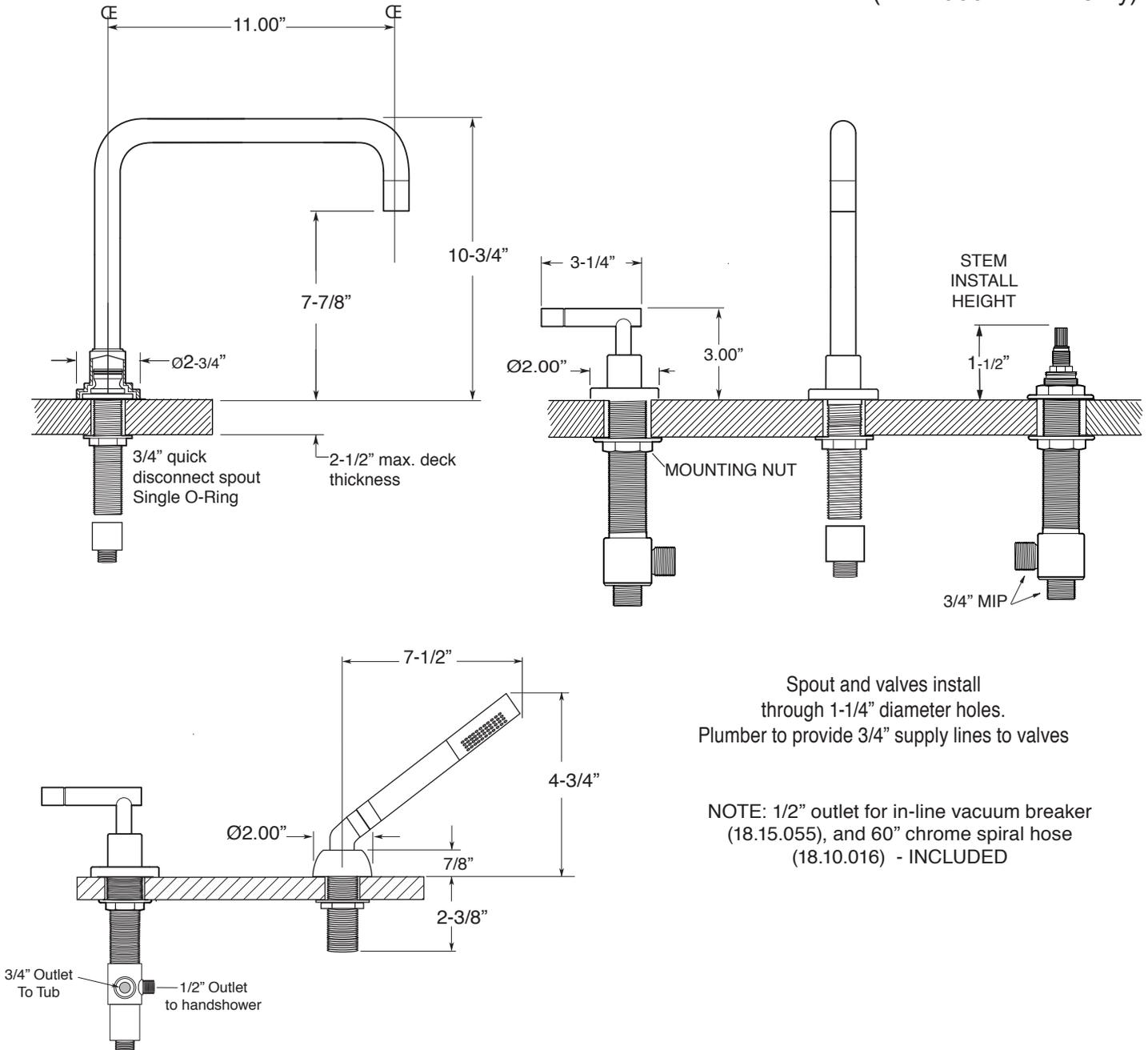
Spout and valves install through 1-1/4" diameter holes.
