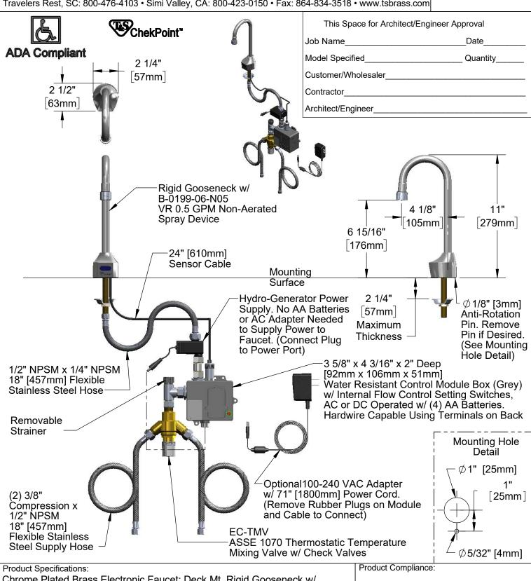
Chrome Plated Brass Electronic Faucet: Deck Mt. Rigid Gooseneck w/ VR 0.5 GPM Non-Aerated Spray Device, AC/DC Control Module w/ Internal Flow Control Setting Switches, Thermostatic Temperature Control Mixing Valve w/ Check Valves, Hydro-Generator, 18" Flexible Stainless Steel Supply Hoses
