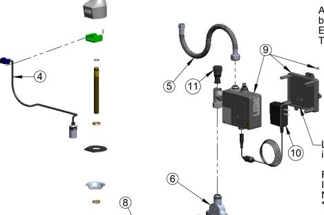
A Maximum of (8) ChekPoint Faucets can be Hardwire Connected and Powered by EC-HARDWIRE ChekPoint Hardwire AĆ Transformer. (Sold Separately)
