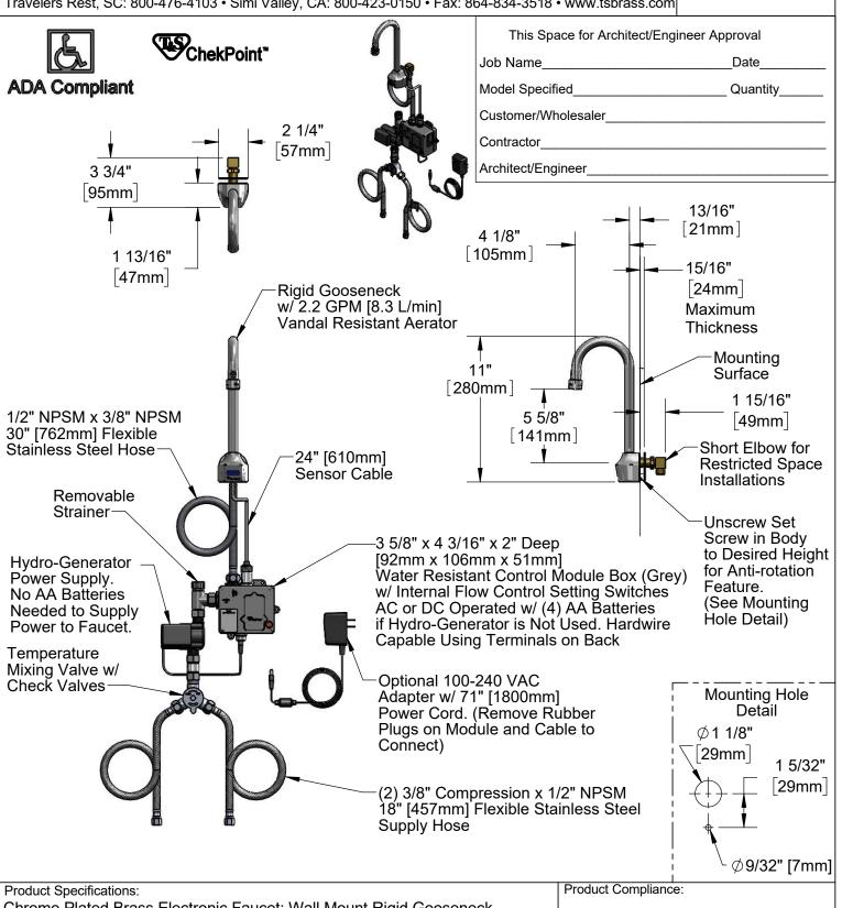
Chrome Plated Brass Electronic Faucet: Wall Mount Rigid Gooseneck w/ 2.2 GPM VR Aerator, AC/DC Control Module w/ Internal Flow Cont. Setting Switches, Temperature Control Mixing Valve w/ Check Valves, Hydro-Generator, 18" Hot & Cold Supply Stop Flexible Connector Hoses
