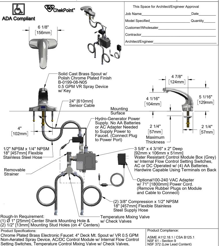
Hydro-Generator, 18" Flexible Stainless Steel Supply Hoses
