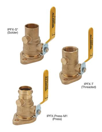
\*This valve is designed to be soft soldered into lines without disassembly, using a low temperature solder to 420°F (216°C). Higher temperature solders may damage the seat material.
